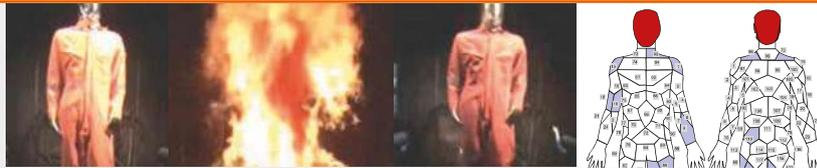
This test method provides the general principles for evaluating the performance of complete garments or protective clothing ensembles in a flash fire or other short duration exposures.
